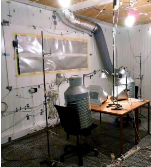
Figures. Experimental chamber with PCM radiant ceiling (left) and PV/T panels (right).
