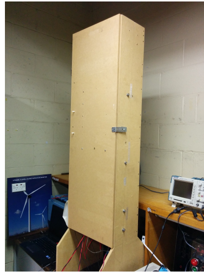
(b) Open ended chimney during thermal measurements
