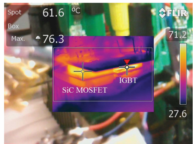
(b) Case temperatures of SiC MOSFET and 600 V IGBT+Diode at 30 kHz and 3 kW
