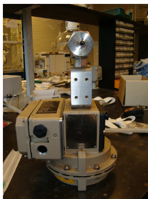
Figure 2.11: Pressure Regulating Valve Figure 2.12: Pressure Valve Actuator
