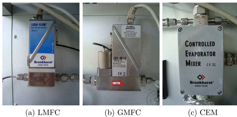
Figure 2.9: Flow Controllers and CEM
