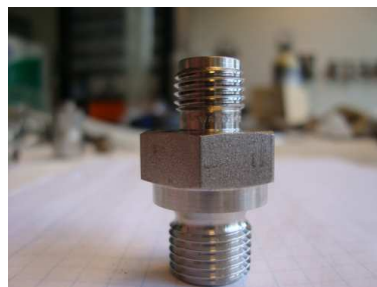
Figure 2.19: Adaptor used to connect the Pressure Valve to the Swagelok Components in the rest of the System
