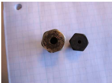
Figure 2.15: Comparison of the K_{vs} values. Left: 0.001 Right: 0.00063
