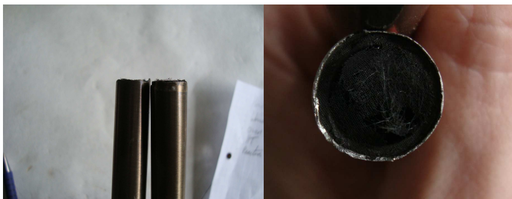
Figure 2.4: Reactor Cross Section and Bed
