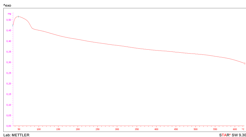
Figure 5.2: Decomposition of \text{RhCl}_3 \cdot x\text{H}_2\text{O}
