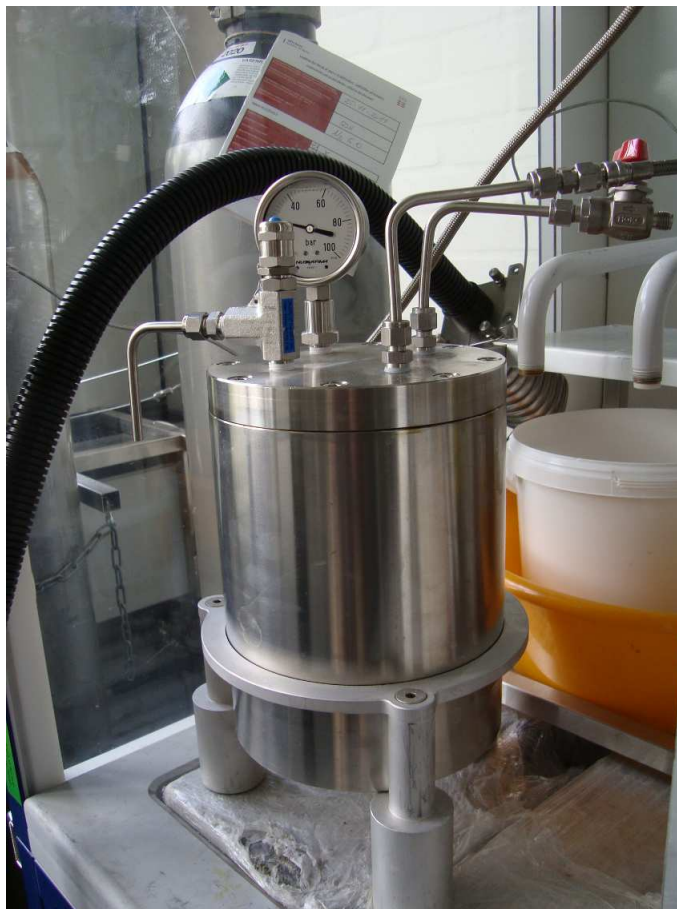
Figure 6.3: MeOH tank used
