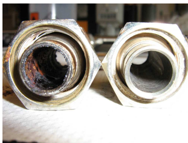
Figure 2.7: Comparing Components Before and After the Reactor
