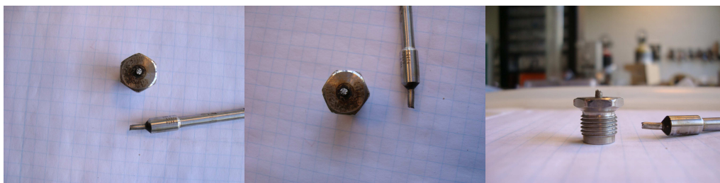
Figure 2.17: Broken Valve Pin
