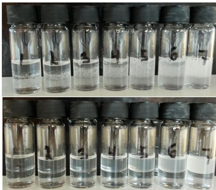
Figure 6.9: Visual turbidity investigations of various BA loadings in undecane, to identify optimal BA loading. The BA concentration increases from left to right, both top and bottom ([0.5; 0.75; 1.0; 1.25; 1.5; 2.0; 3.0] M BA in undecane, respectively). The top picture also indicates that a lower BA concentration reduces the time needed for achieving phase splitting.
