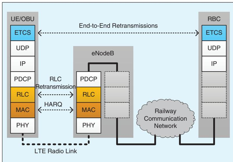
**FIGURE 2** A simplified LTE protocol stack. Three available retransmission mechanisms are shown at the MAC layer, at the RLC layer, and at the application layer (i.e., ETCS layer). PDCP: packet data convergence protocol. IP: Internet protocol.
