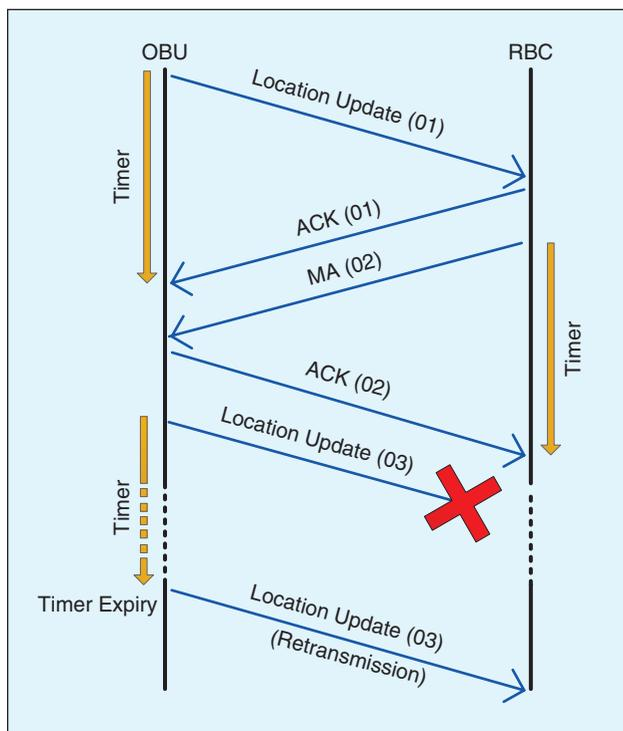
**FIGURE 3** An example of an ETCS OBU–RBC message exchange with the end-to-end retransmission mechanism. The first two messages (location update 01 and MA 02) are delivered successfully before their retransmission timers expire. The third message (location update 03) is lost by the underlying transport network and does not arrive at the RBC. When the retransmission timer at OBU node expires, the location update 03 message is retransmitted.
