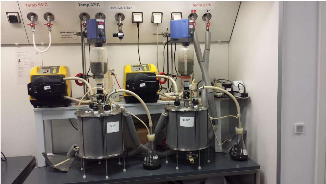
Figure S3 – Experimental set-up for the co-digestion process in a continuously stirred tank reactor.
