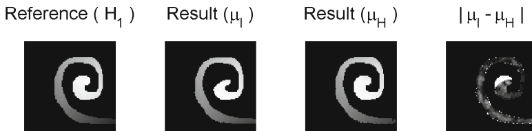
Fig. 4. Registration results on the synthetic 2D data. From left to right: The reference heat distribution H_1 , The moving heat map, H_2 , after transformation using the registration results, i.e. H_2(T_{\mu_I}) and H_2(T_{\mu_H}) . Finally, the difference between the results, i.e. |H_2(T_{\mu_I}) - H_2(T_{\mu_H})| .
