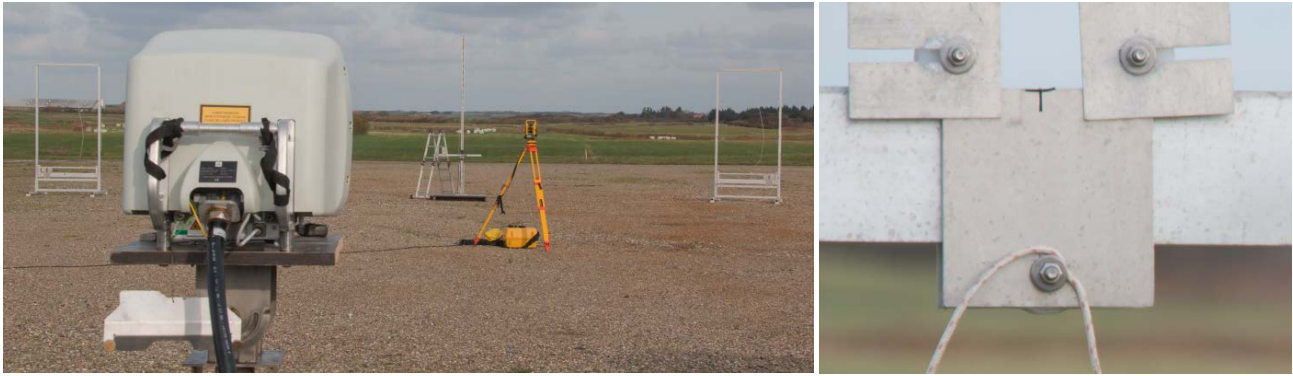
Figure 4. Left: photograph of the measurement setup for ground calibration of the 5-beam Demonstrator's inclinometers. Right: shutters for detecting the beam position by blocking/unblocking
