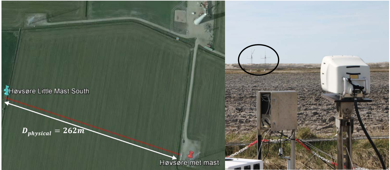
Figure 15. Calibration measurement setup of the AVENT 5-beam Demonstrator lidar at DTU Wind Energy test site, Høvsøre (DK)
