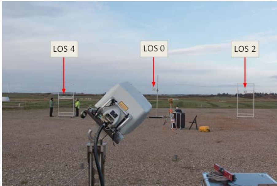
Figure 13. Photograph of the measurement setup for geometry verification of the 5-beam Demonstrator
