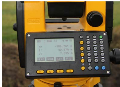
Figure 5. 3D coordinates measurements with a theodolite
