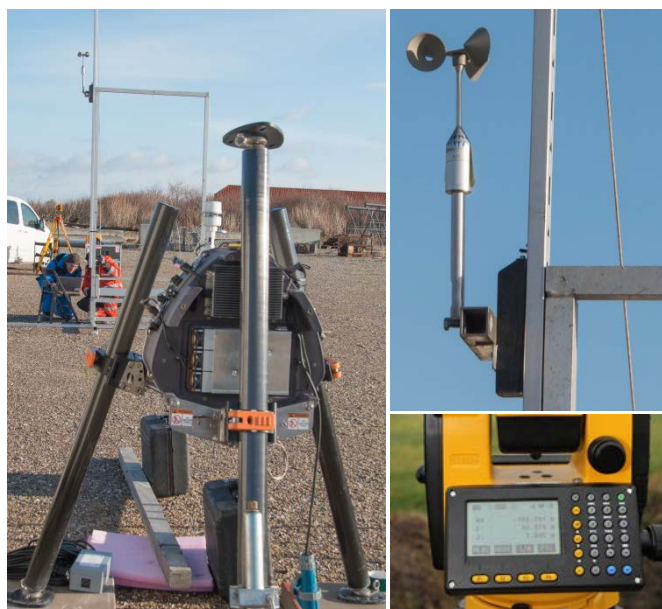
Figure 5. Left: photograph of the measurement setup for ground calibration of the ZephIR Dual-Mode tilt inclinometer. Top right: cup anemometer used as moving hard target. Bottom right: 3D coordinates measurements with a theodolite
