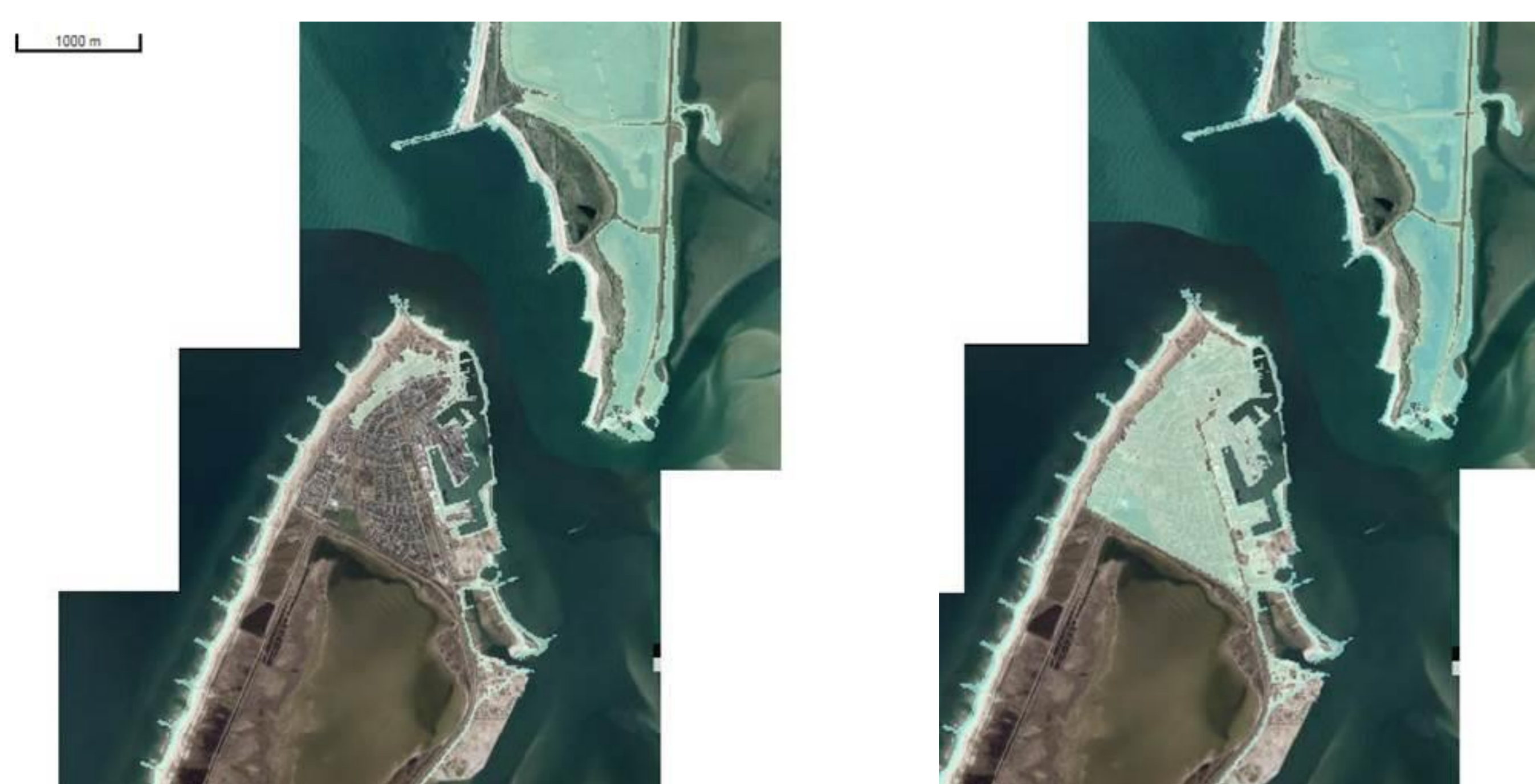
Figure 5. Potential flooding extent from a storm surge at Thyboron Harbor with a return period of 50 years in 2016 (left) and in 2060 including sea level rise and land subsidence.
