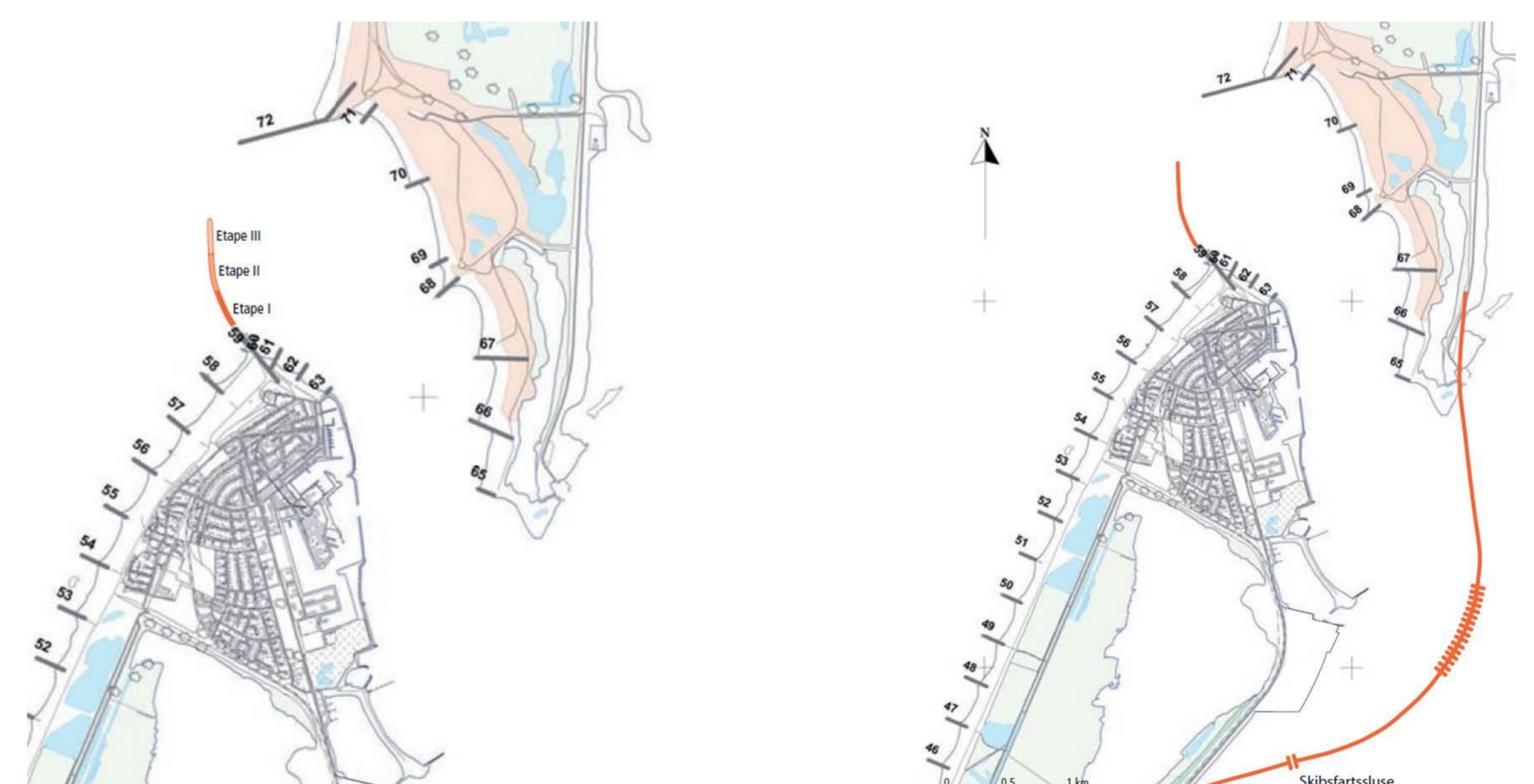
Figure 6. Technically preferred management option: extending a groin to a breakwater (left) and an alternative management option with a sluice.
