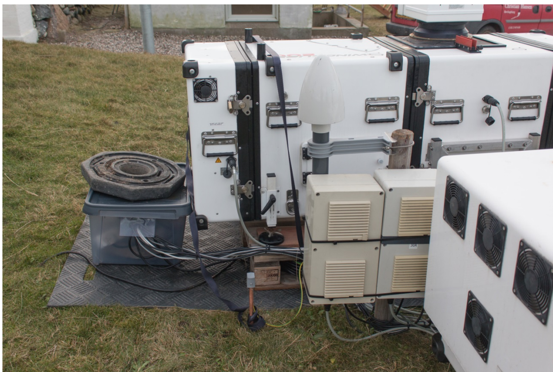
Figure 24 Details of the RUNE2 installation showing the power supplies, GPS antenna, earthing pole and communications box.
