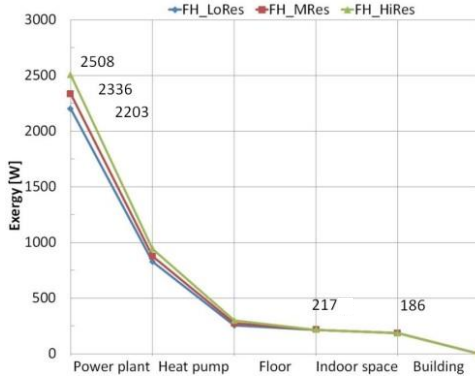
Fig. 3 Exergy flows for the floor structures with different floor covering resistances, heating
