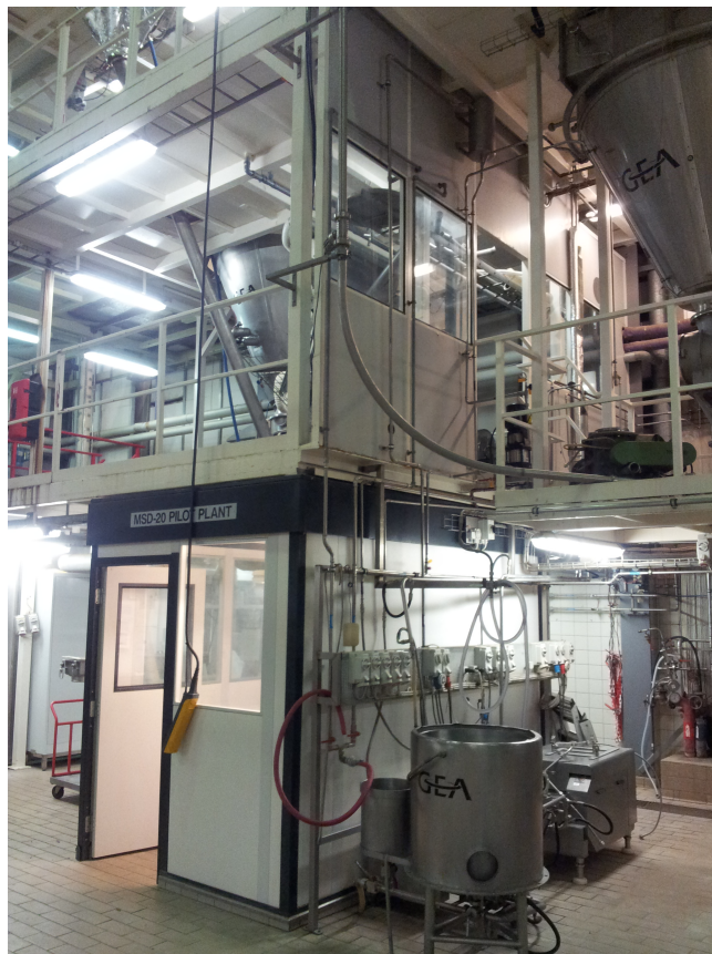
Figure 2.2: The picture of the MSD TM -20 spray dryer seen from the ground floor.
