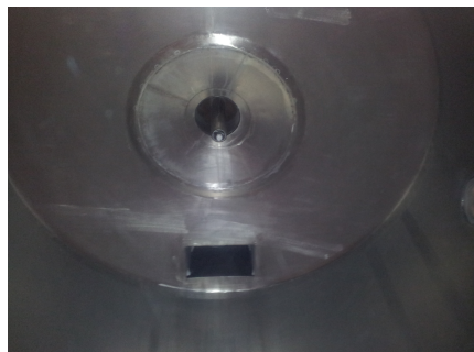
(a) The SD stage with nozzle and exhaust air outlet.
