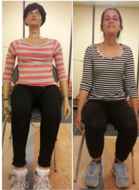
Figure 7.2 The outlook of the thermal manikin and a real human subject.
