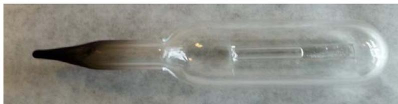
**Figure 2.** Photograph of a sealed ampoule with a small amount of water/ice contained inside a capillary. This ampoule contained water and 0.5 bar of hydrogen. The carbon sooting (on the outside) helped avoiding crack formation in the glass after sealing.
