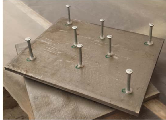
Figure 8.6 Cast-in element with powder actuated nails
