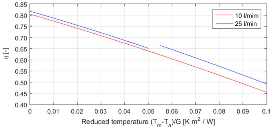
Fig. 1. Soleff efficiency curves for the HT-SA collector at 45° tilt angle and an hemispherical irradiance of 1000 W/m<sup>2</sup>.
