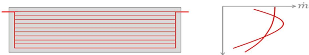
Fig. 2. Example flow distribution in a harp collector [11].
