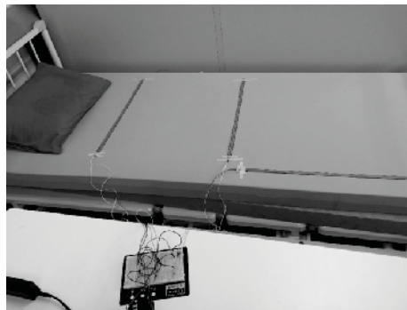
Figure 2. Developed sensing system to prevent bed-related accidents.
