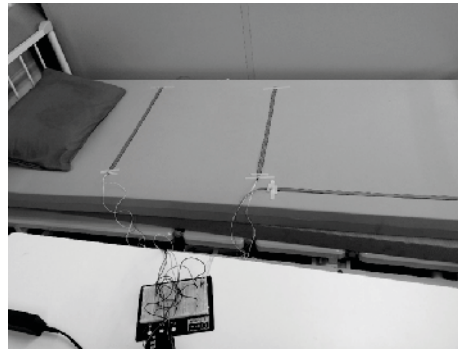
Figure 2. Developed sensing system to prevent bed-related accidents.
