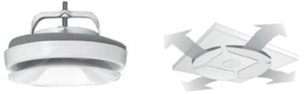
Figure 4: Investigated non-motorized diffuser. Left figure: Circular air diffuser with fixed opening area. Right figure: Active air diffuser with self adjusting inlet vanes that changes the outlet area depending on the pressure upstream of the diffuser
