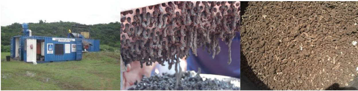
Figure 5 Prototype of the LaDePa machine in an old container (left), pasteurised faecal sludge (middle), and hygienised end product (right) (pictures: Günter Langergraber).
