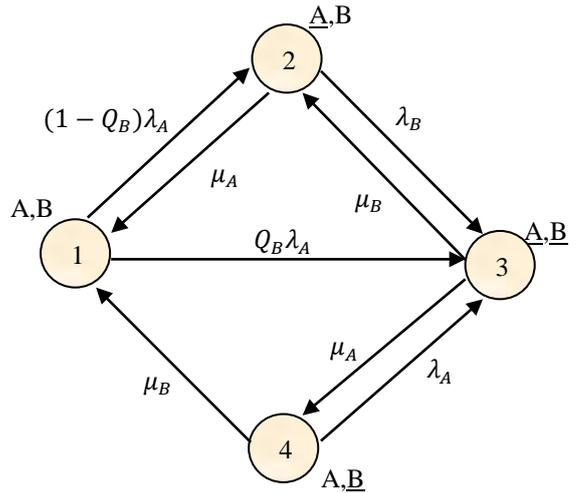
Figure 2. State diagram of the power supply system
