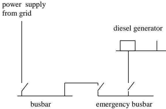
Figure 1. System layout of the power supply system
