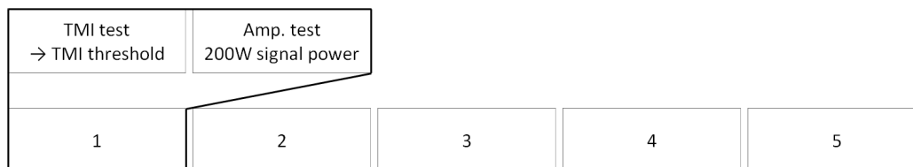
Figure 6. The following test procedure consists of 5 tests each including a TMI test and an amplifier test, where the DMF rod fiber is operated as an amplifier delivering 200 W of signal average power for 6 h - 8 h.
