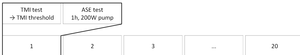
Figure 4. The initial test procedure consists of 20 tests, where one test include a TMI test and one ASE test, performed on the DMF rod fiber.
