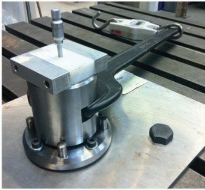
Figure 7. Left: setup for tool compression and inner broach diameter measurements; right: graph of experimental, analytical and numerical inner broach diameter compression as a function of torque.
