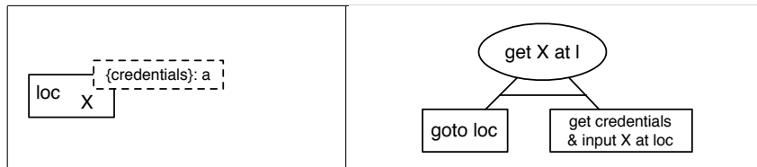
Fig. 5. To obtain an asset from a location, the transformation generates the necessary attack to go to the asset’s location, then obtains the credentials, and finally performs the necessary in action.
