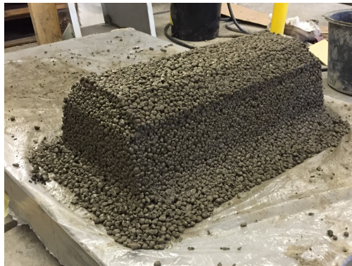
(a) LWAC block immediately after casting. Immediately after removal of the mold, the block was covered in three layers of plastic.
