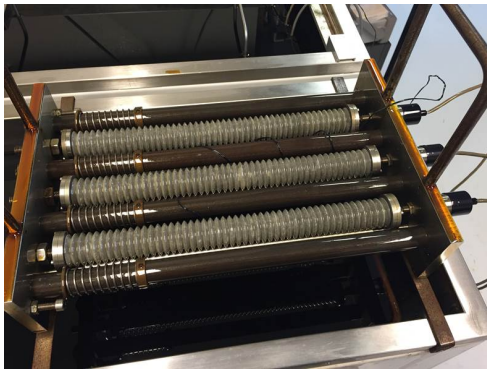
Figure 7: Test setup for the automatic dilatometer test for expansion measurements of mortars during the first 28 days after mixing. A displacement transducer measured the deformation in one end of each of the specimens. During testing, the specimens were immersed in a thermo-bath filled with polyalkylene glycol at a constant temperature of 20°C.
