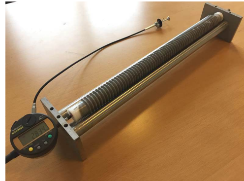
Figure 8: Test setup for manual dilatometer test for expansion measurements of mortars during the first hour after mixing. The deformation was read from a digital length gauge at one end of the specimen.
