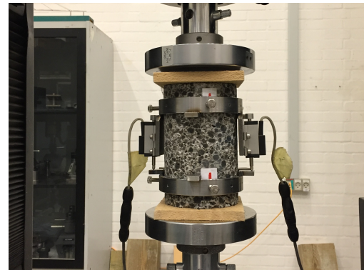
(b) Test setup for strain measurements of LWAC. Two rigid rings were each tightly fastened to the specimen with three screws, and two extensometers were placed between the rings on opposite sides.
