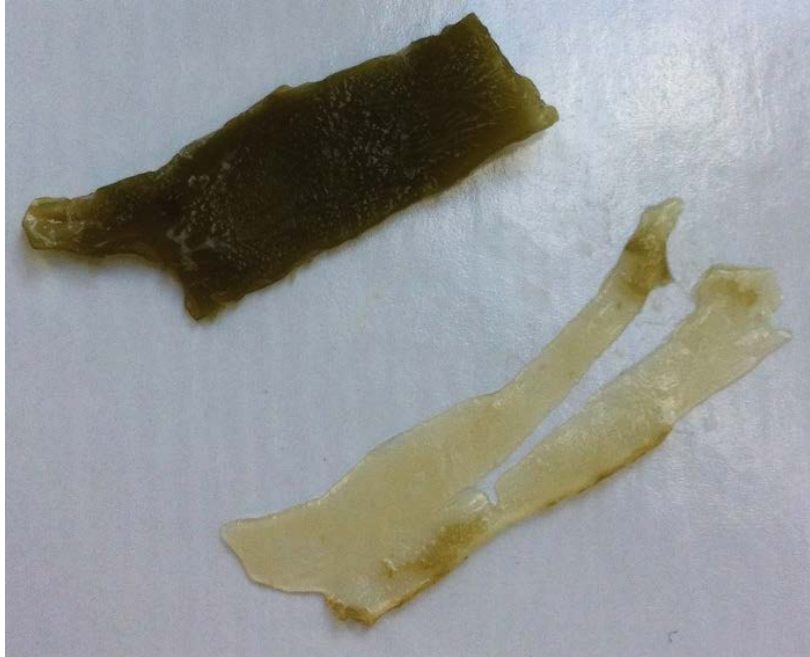
Figure 15: Pretreated (wet refiner milling at disc distance 2.0 mm) Laminaria digitata . Top: before enzymatic treatment. Bottom: after 90 min of enzymatic treatment with the cellulase preparation Cellic®CTec2 (Novozymes) and alginate lyase (Sigma Aldrich).
