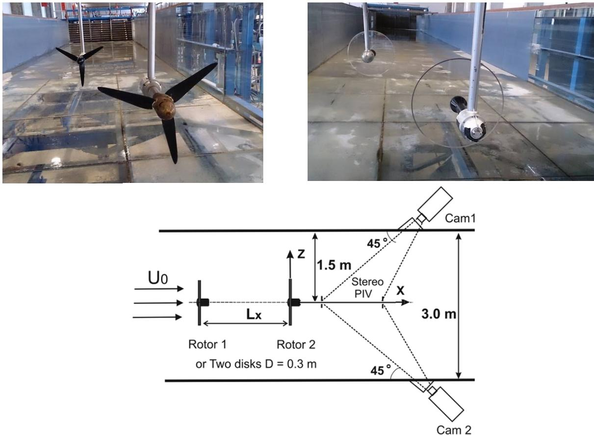
**Figure 1.** Photos and sketches of the experimental setup.
