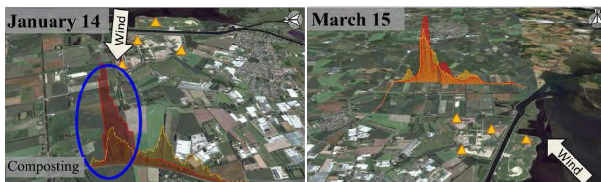
Figure 1. Methane (red) and tracer gas (yellow) plumes measured downwind of the landfills. The orange triangles indicate the tracer gas release locations.
