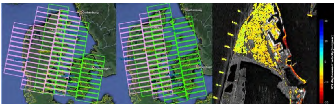
Figure 1 S-1 coverage over Denmark in ascending and descending tracks, and subsidence map over Thyborøn where orange and red colors indicate subsidence and green relative stability (right).
