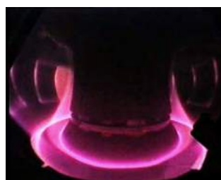
The ASDEX Upgrade fusion device, with hot plasma glowing in pink
