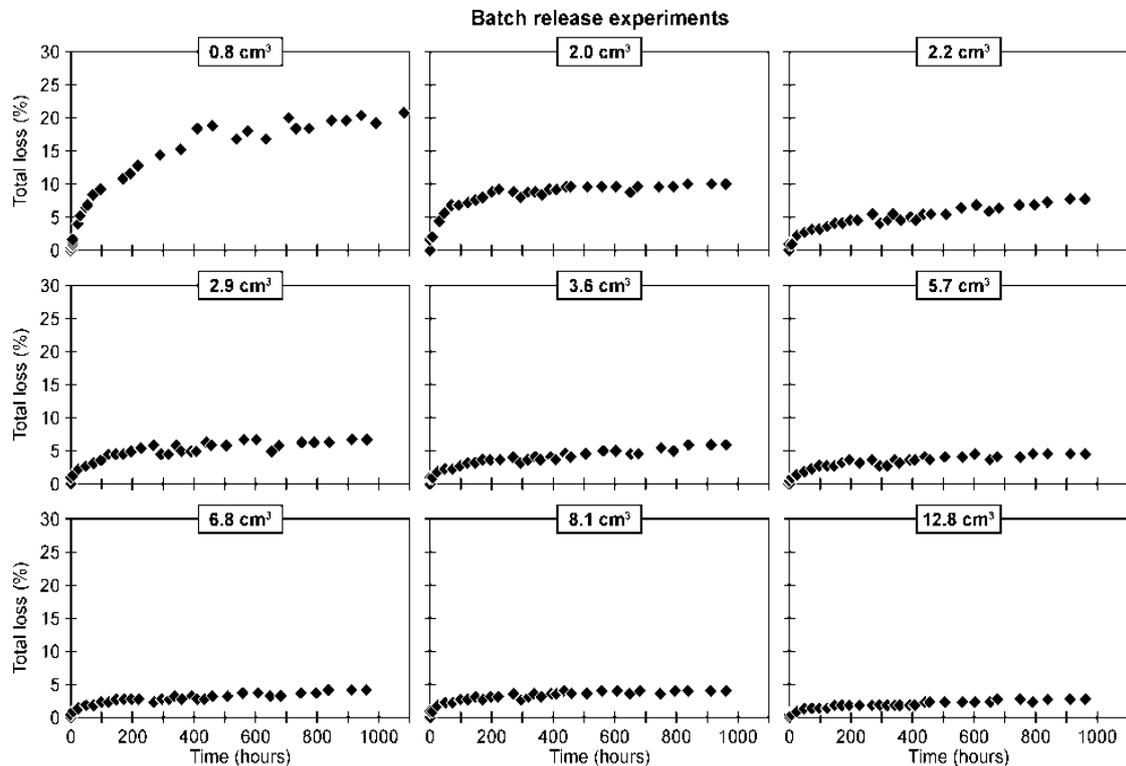
Figure 1. The time dependency of the total loss of HCFC-141b in percentage of initial content from foam particles with different sizes (Kjeldsen and Scheutz 2003).
