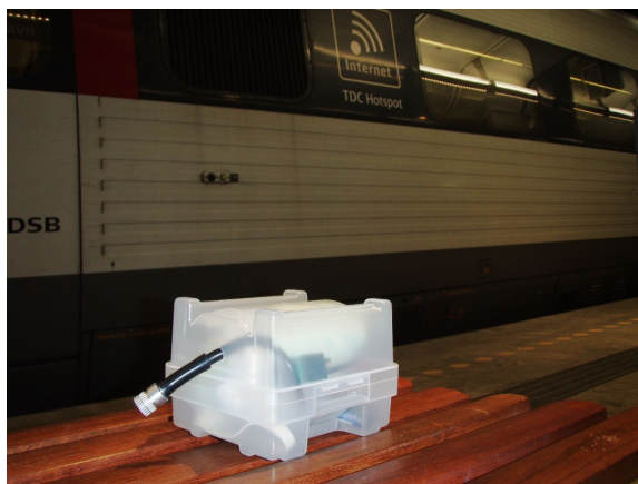
Figure 9.4: Field sampling at Nørreport station in Copenhagen. The sampling box consists of an impactor to remove particles larger than 500 nm, a deposition chamber where a chip with strings is placed, and a battery-driven pump.
