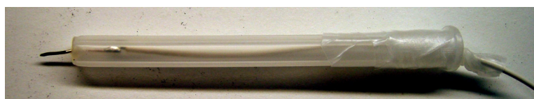
Figure 2.7: Quasi Ag/AgCl electrode fabricated from a Ag wire.
