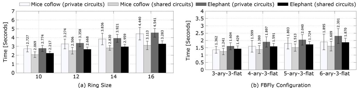
**Figure 5: Average completion time of mice coflows and elephant flows under *intensive* network load, over two upper tier topologies: (a) Ring (10 to 16 packet switches) and (b) FBFLy (9 to 36 packet switches).**
