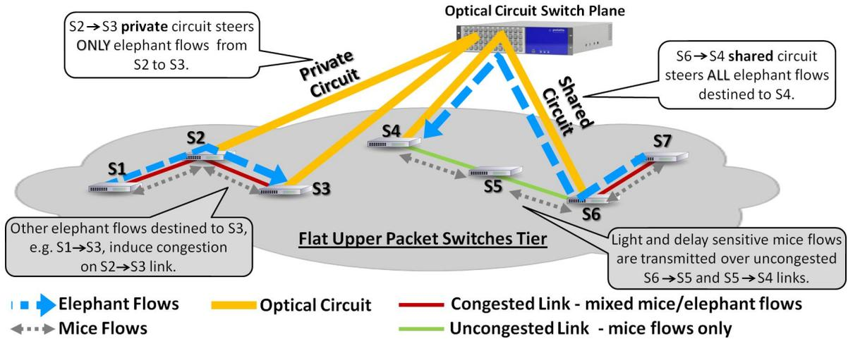
**Figure 1: The *C-Share* topology concept. *Private* optical circuit results in inefficient mice/elephant flow separation over  $S2 \rightarrow S3$  link. On the other hand, a *shared* optical circuit reduces the load over  $S6 \rightarrow S5$  and  $S5 \rightarrow S4$  links by better mice/elephant flow separation.**
