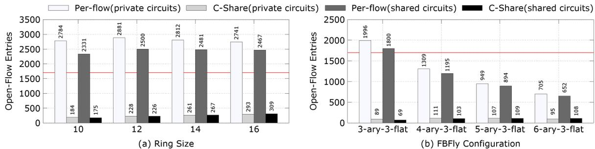
**Figure 6: OpenFlow rule footprint per switch during one minute of network trace under *intensive* network load, over two upper tier topologies: (a) Ring (10 to 16 packet switches) and (b) FBFLy (9 to 36 packet switches). The horizontal line indicates 1.7k OF rule entries. Any OF entries count above it might be an unfeasible scenario.**
