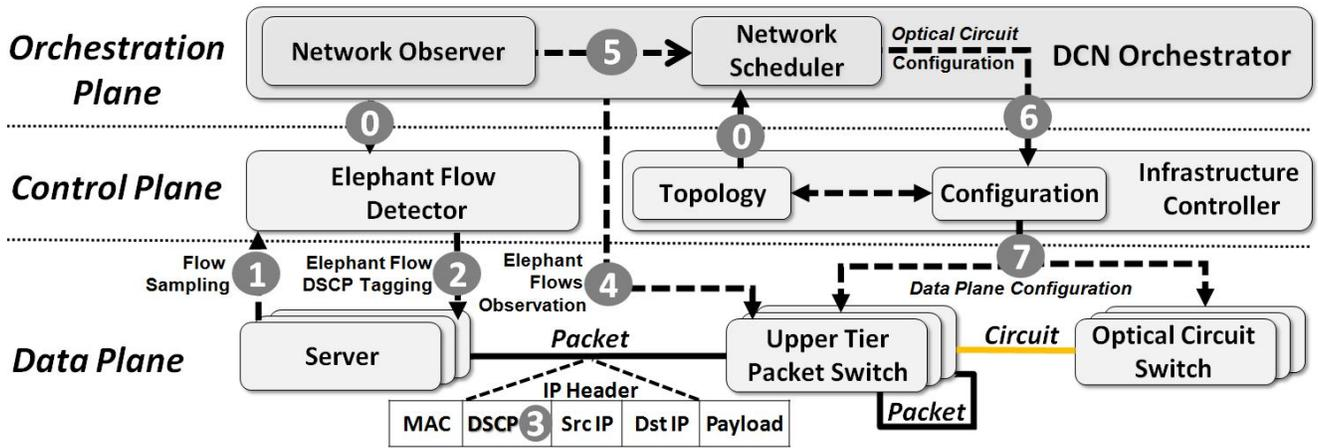
Figure 2: *C-Share* architecture block diagram and workflow.
