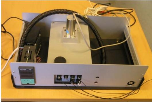
**Figure 1.** External view of the light-tight box containing the microfluidic cartridge. The photomultiplier shown in the picture is placed perpendicular to the surface of the cartridge and the collected signal is transmitted to a PC.
