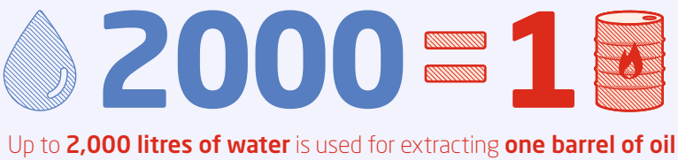
Oil extraction consumes from 500 to 1,200 litres per MWh, corresponding to about 800 to 2,000 litres for one barrel. Coal extraction employs water consumption rates of 15 to 105 litres per MWh for mining and washing, and an additional consumption of 40 to 90 litres per MWh if transported by slurry pipeline.
