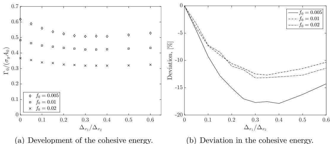
Figure 3: Mode I-Mode III analysis for varying ratios of  $\Delta_{x_1}/\Delta_{x_2}$ . The deviation is calculated as  $(\Gamma_{0,\Delta_{x_1}/\Delta_{x_2}} - \Gamma_{0,Mode I})/\Gamma_{0,Mode I}$ .
