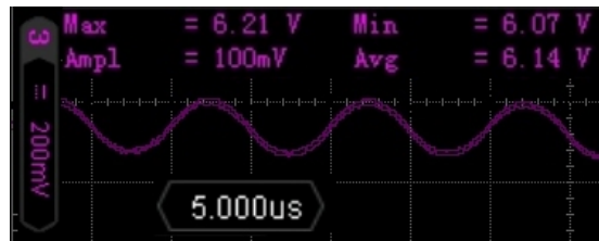
Fig. 7. Output ripple at 50% duty cycle with 2.5\Omega
