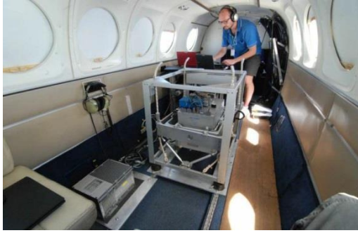
Figure 2. The Imar-IMU unit and LCR S-99 gravimeter.
