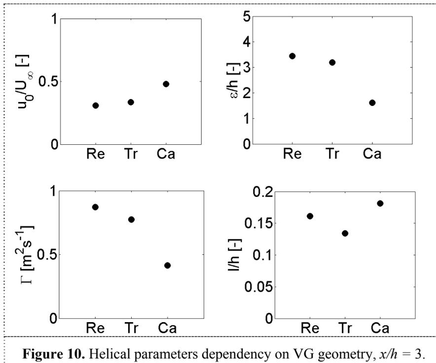
Figure 10. Helical parameters dependency on VG geometry,  $x/h = 3$ .
