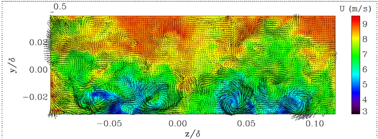
**Figure 4.** Example of instantaneous velocity field,  $x/h = 12$ .
