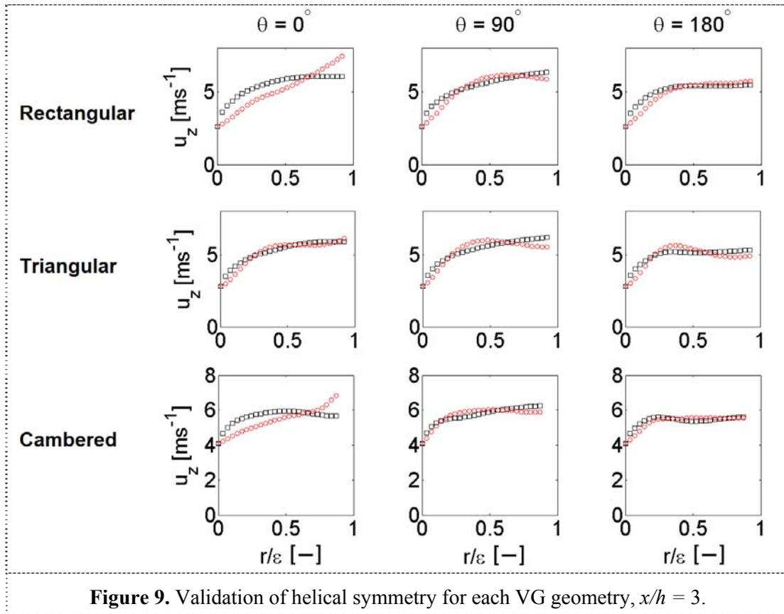
Figure 9. Validation of helical symmetry for each VG geometry,  $x/h = 3$ .
