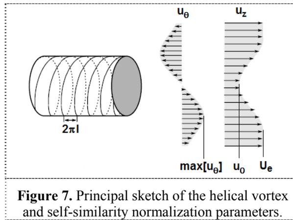
**Figure 7.** Principal sketch of the helical vortex and self-similarity normalization parameters.
