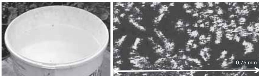
Figure 1. Carbonation on the surface of limewater. Crystals can be seen in the microscope.
