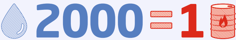
Oil extraction consumes from 500 to 1,200 litres per MWh, corresponding to about 800 to 2,000 litres for one barrel. Coal extraction employs water consumption rates of 15 to 105 litres per MWh for mining and washing, and an additional consumption of 40 to 90 litres per MWh if transported by slurry pipeline.
