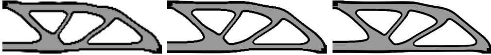
Figure 8: Optimized MBB beam. Left: 150 by 50 elements ( c = 324.3 ). Middle: 300 by 100 elements ( c = 305.2 ). Right: 600 by 200 elements ( c = 305.8 ).
