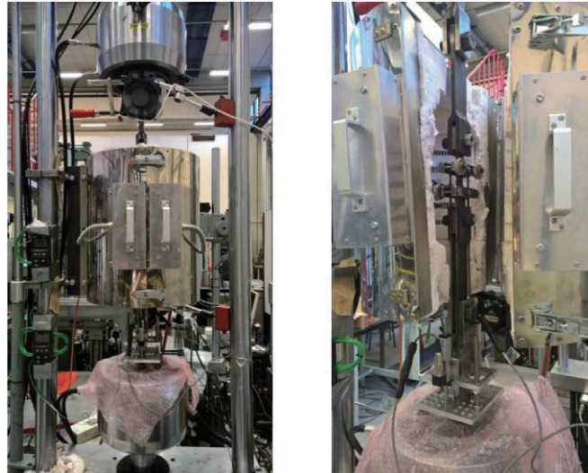
Fig. 1: High temperature monotonic tensile test setup.
