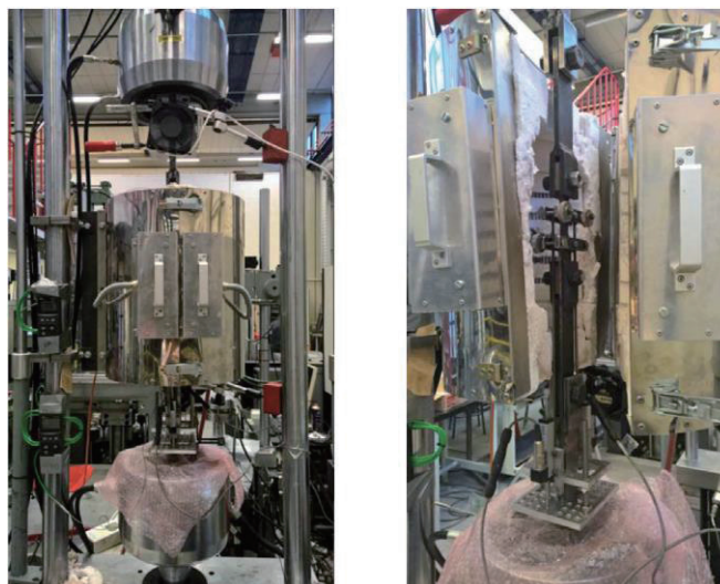
Fig. 1: High temperature monotonic tensile test setup.
