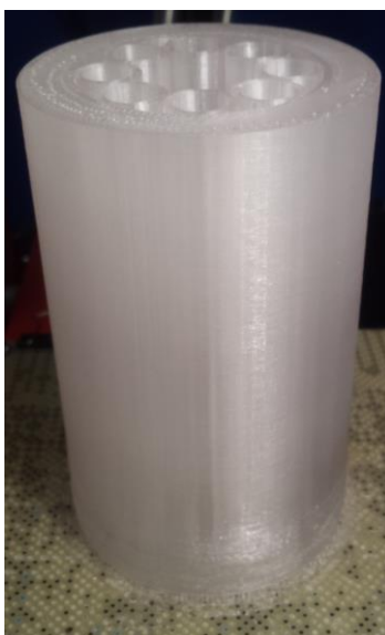
Figure 2. Hollow-core PMMA mPOF preform on the printing bed.
