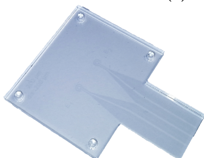
(b) Chip substrate with printed electrodes
