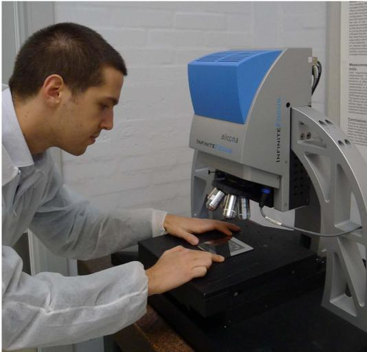
In connection with the use of brass specimens featuring structured surfaces in a tribology test, an algorithm was developed for automatic measurement of the contact area by optical means.
