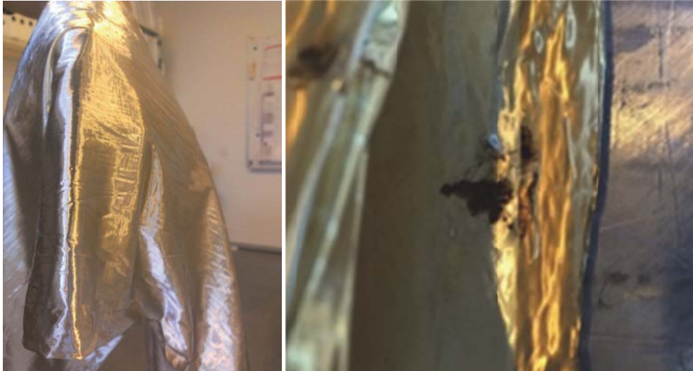
Figure 27 - DEAP-film (a) a piece of DEAP film (b) a piece of DEAP film with breakdowns [right photo: Emmanouil Dimopoulos]
