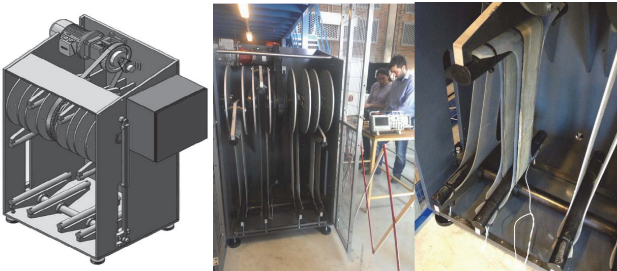
Figure 38 - (left) CAD drawings of demonstrator, (middle) picture of the built demonstrator used as demonstrator 1, 2, and 3, and (right) the DEAP Linear transducers attached to the machine [left figure: CAD from project material, right photo: Emmanouil Dimopoulos]
