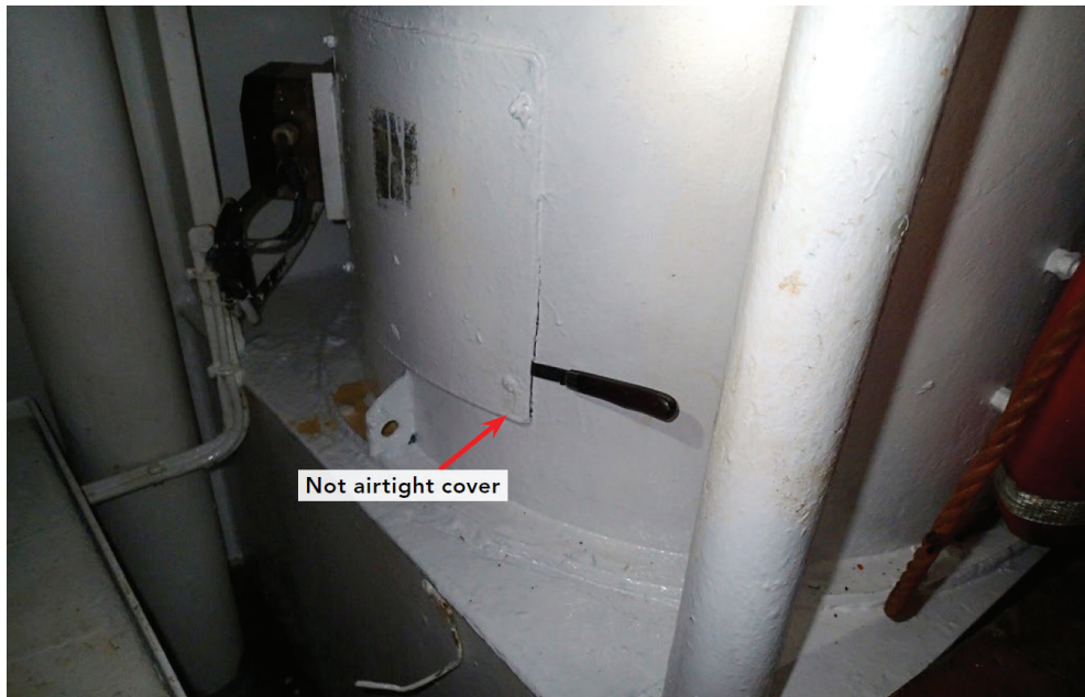
Figure 2. The inspection hatch on a ventilation duct that ran from the cargo hold through the forecabin. A minor gap in a section of the rim (knife blade inserted) allowed gasses to travel from the cargo hold to the bow area. (LADY IRINA). Source: [13].
