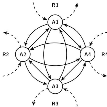
Figure 8: The *complete* transshipment structure shown for a physical port,  $A$  with four rotations visiting the port.  $A1$ ,  $A2$ ,  $A3$ , and  $A4$  are the corresponding port calls. Solid edges correspond to transshipment edges and dashed to voyage edges for the four different rotations visiting port  $A$ .
