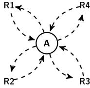
Figure 6: Simple transshipment structure shown for a physical port,  $A$ , with four rotations visiting the port. Voyage edges are dashed and cargo transshipment directly from one voyage edge to another.
