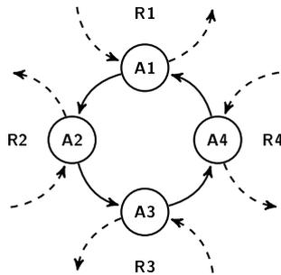
Figure 7: The transshipment structure shown for a physical port,  $A$  with four rotations visiting the port.  $A1$ ,  $A2$ ,  $A3$ , and  $A4$  are the corresponding port calls and they are connected in a ring. Solid edges correspond to transshipment edges and dashed to voyage edges.
