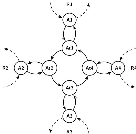
Figure 10: The *ring* transshipment structure shown for a physical port,  $A$  with four rotations visiting the port.  $A1$ ,  $A2$ ,  $A3$ , and  $A4$  are the corresponding port calls.  $At1$ ,  $At2$ ,  $At3$ , and  $At4$  are extra transshipment nodes. Solid edges correspond to transshipment edges and dashed to voyage edges for the four different rotations visiting port  $A$ .
