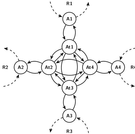
Figure 11: A general transshipment structure shown for a physical port,  $A$ , with four rotations visiting the port.  $A1$ ,  $A2$ ,  $A3$ , and  $A4$  are the corresponding port calls.  $At1$ ,  $At2$ ,  $At3$ , and  $At4$  are extra transshipment nodes and edges are added between all pairs of these. Solid edges correspond to transshipment edges and dashed to voyage edges.
