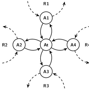
Figure 9: The *star* transshipment structure shown for a physical port,  $A$  with four rotations visiting the port.  $A1$ ,  $A2$ ,  $A3$ , and  $A4$  are the corresponding port calls and  $At$  is an extra transshipment node. Solid edges correspond to transshipment edges and dashed to voyage edges for the four different rotations visiting port  $A$ .
