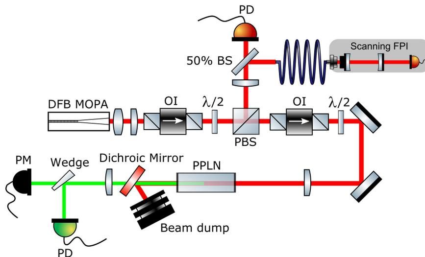
Figure 1. The setup. OI: Optical Isolator,  $\lambda/2$ : Half wave plate, PBS: Polarizing beam splitter, BS: Beam splitter, PD: Photodiode, FPI: Fabry-Pérot interferometer, PM: Thermal power meter, PPLN: 50 mm periodically poled lithium niobate.
