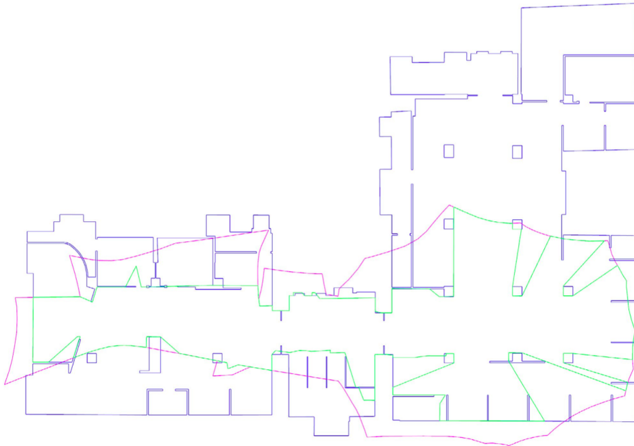
Figure 34.: Area covered by CCTV cameras after radial distortion correction (purple) and taking into account the topology of the building (green)
