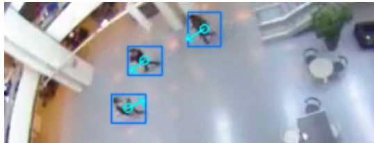
Figure 13.: Three principals described by bounding boxes. The arrow indicates the median flow.
