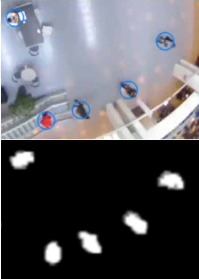
Figure 3.: Background segmentation. For each pixel in the image a label w is inferred denoting the absence or presence of a foreground object.
