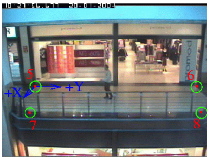
Figure 25.: Lisbon ground plane homography for view (b)
