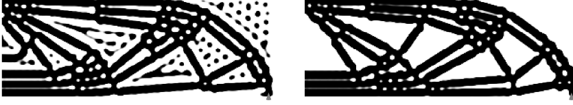
Figure 15: MBB beam designs with maximum length scale imposed on both phases (left) and only on the solid phase (right).
