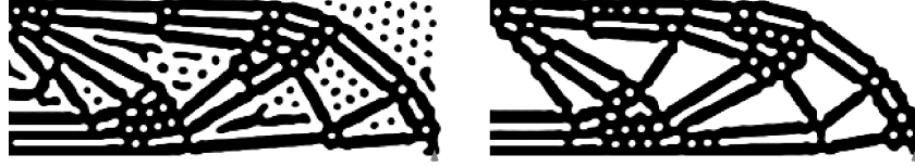
Figure 16: MBB designs with minimum and maximum length scale imposed on both phases (left) and maximum length scale only on the solid phase (right).
